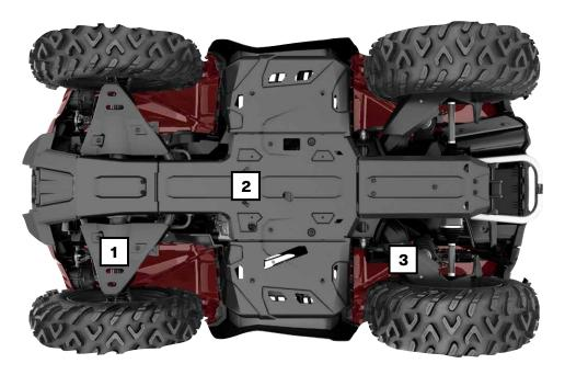
Our plastic plates glide smoothly and silently over obstacles, offering great protection in rough terrain. Made of 1/4" (6 mm) thick abrasion-resistant thermoformed high molecular weight polyethylene (HMWPE).
